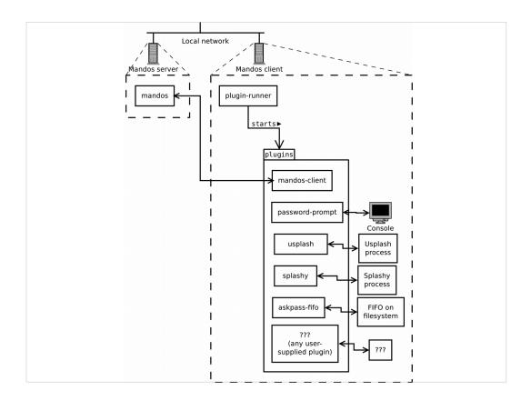
Client-side process model with plugins for various input methods, etc.
