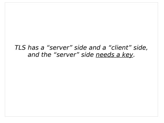
A fundamental property of TLS is the the server side absolutely needs a key, and the client side key is merely optional. The TLS key can be a X.509 certificate
