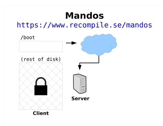
The encrypted server's unencrypted part runs code which locates a server on the network, and connects to it.
